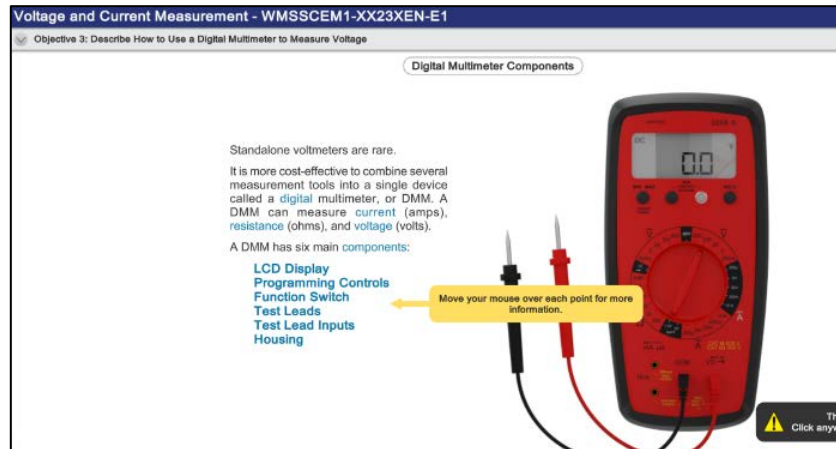
Figure 23: Components of a digital multimeter
